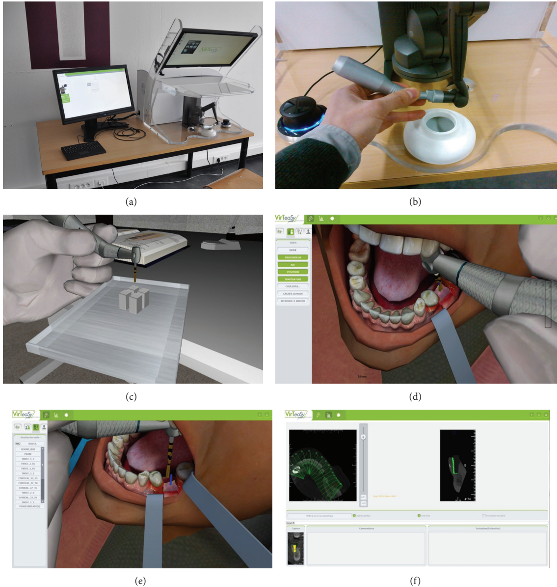
FIGURE 1: Haptic simulator and virtual exercises. (a) Overview of the simulator. (b) Positioning of the haptic contra-angled handpiece. (c) Image of the virtual drilling procedure. (d) Virtual implant site preparation. (e) Blue angulation guide. (f) Grading of virtual drilling (green is reference and black is actual drilling).
